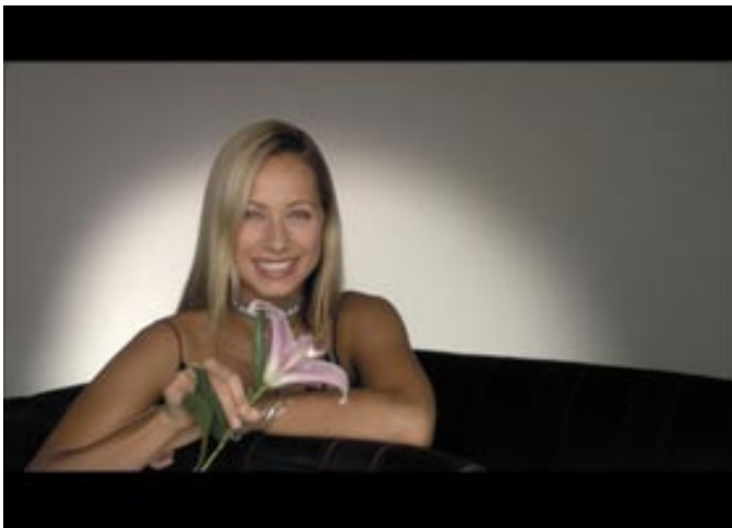
Figure 3 – 16:9 image anamorphic squeezed into a 4:3 screen area
